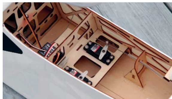
There's plenty of room for your radio components in this fuselage. I had to slightly enlarge the servo openings to accommodate the servos I used.
