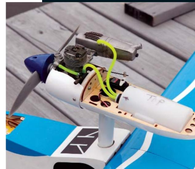
During assembly, setting up the pod's thrust line is extremely important in terms of how straight and level the model will fly—hands-off.
