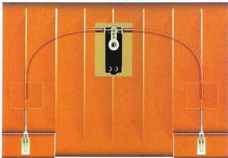
My modified aileron servo installation helps keep the radio dry.
