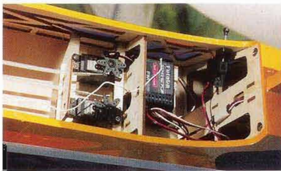
The fuselage structure is laser-cut ply and the radio gear mounts up and away from the cabin floor to withstand the rigors of flying from water.
