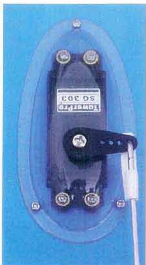
These included clear covers shield the aileron servos from getting splashed.
