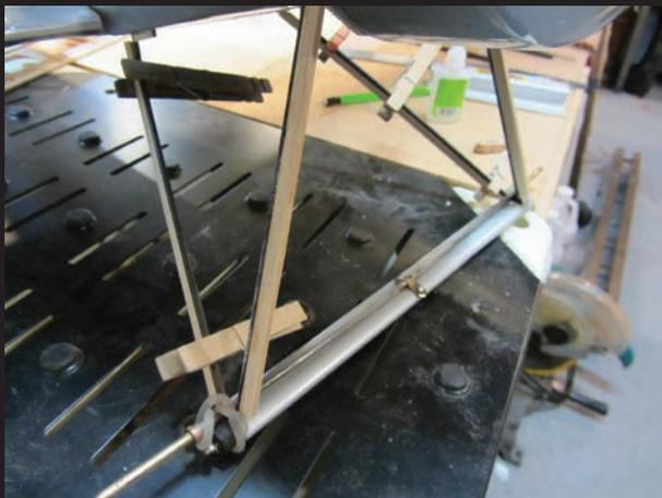
Above: I made some scale strut fairings out of scrap balsa because those that came with the ARF were slightly large.
