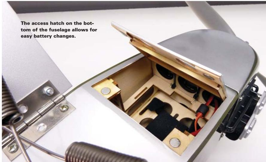
The access hatch on the bottom of the fuselage allows for easy battery changes.
