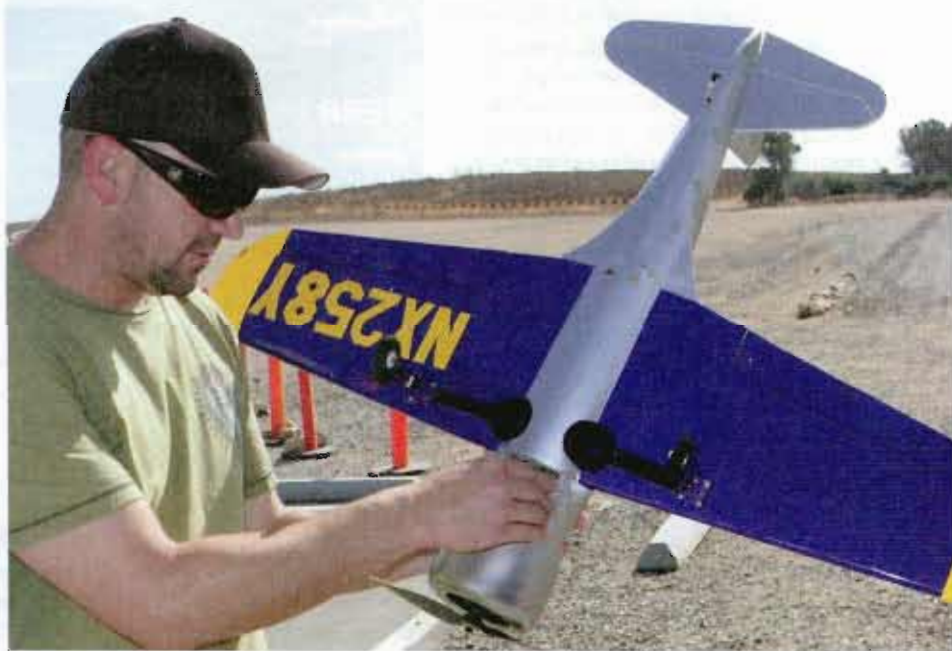
Removing the magnetized hatch allows for fast and easy battery pack swaps. Be sure to pull the hatch toward the nose of the model as to disengage the carbon fiber holding pins while detaching it.
