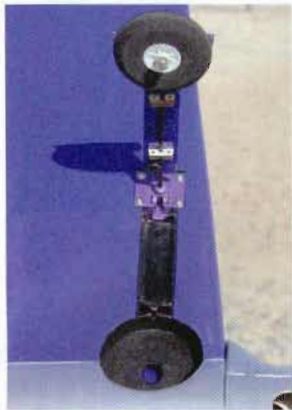
Once set up correctly, the mechanical retracts do the job well and are a nice option for this plane.
