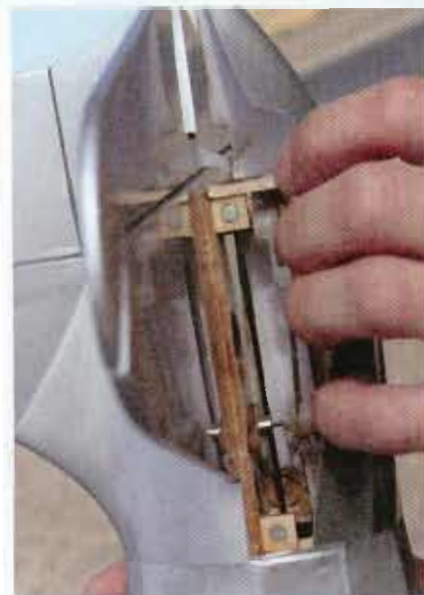
Peeling away the magnetized fairing reveals a look inside the empennage control area.
