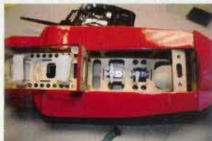
RC bay has ample room for receiver and servos. Note the diligent placement of lightening holes.
