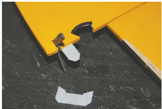
side of the fuse (at left). Some slight bending was required to get the screw holes to line up. The rudder is shown here with its control horn glued in place (below right). Chris added the section of CyA hinge as the bottom of the rudder would be unsupported without it.
