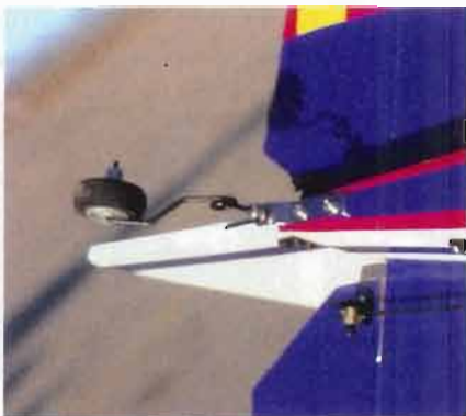
The tailwheel assembly and control hook-up is easy to install and provides plenty of ground authority. Steering is easy for this tail-dragger.
