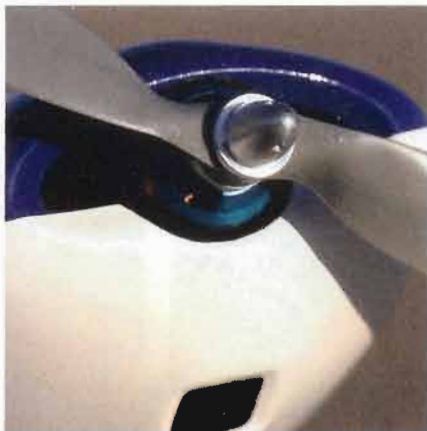
The cowling has plenty of area for cooling. Only a little trimming was necessary for a good fit.
