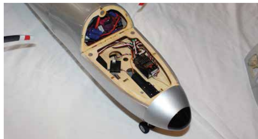
The top hatch provides convenient access to install the dual 4S flight batteries. With everything mounted up front as shown, no weight was required to balance the E-2.
