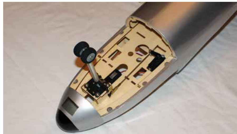
Magnetic hatches provide easy access to install and maintain components such as the nose gear and steering servo shown here.
