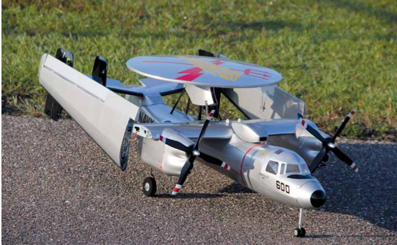
The wings on the full-scale E-2 fold to save precious real estate in the cramped quarters of an aircraft carrier. The Maxford E-2 faithfully replicates that and allows the model to be stored and transported with the wings installed. They can be folded and locked in place for flight in only a few minutes.
