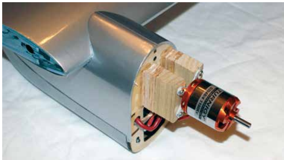
Several blocks are provided to get the proper standoff distance for the dual electric motors. The recommended power system has plenty of power to fly in a scalelike manner, but also to get you out of trouble if you need full throttle.
