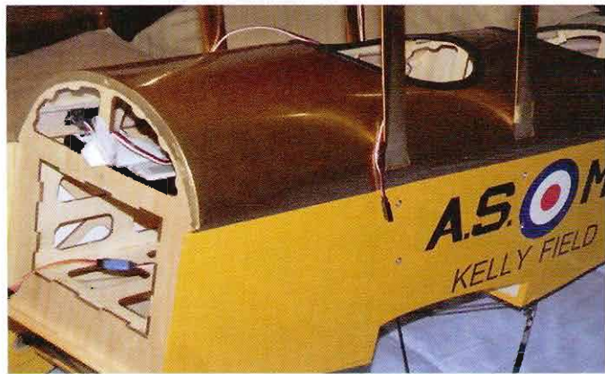
All of the electronic assembly coming together. The "firewall" is not yet installed, allowing easy internal access.
