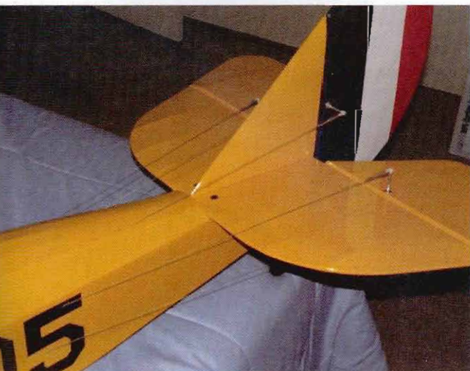
The pull-pull wires for the elevator and rudder come pre-installed from the factory. A nice touch.
