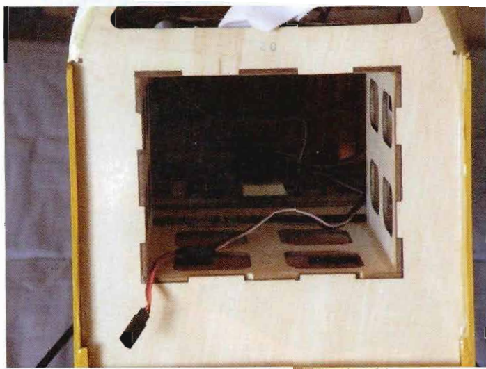
A view from the front showing the elevator and rudder servos plus the receiver. The servo extension wire is for the throttle.
