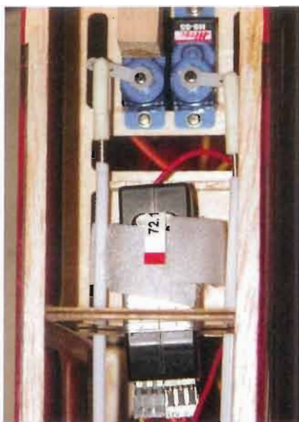
The radio compartment has plenty of room for the servos and receiver.
