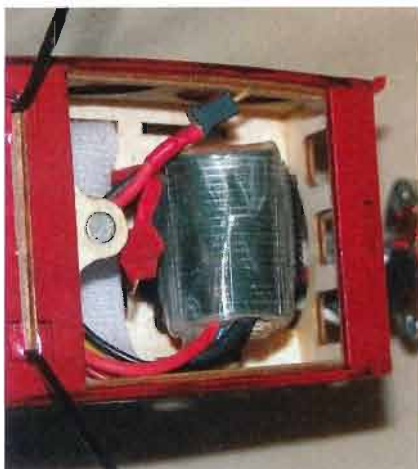
The main gear is held in place with a friction plate and the battery cover is held in place with a tiny magnet.
