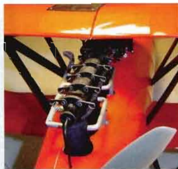
The dummy in-line engine really looks the part, right down to the valve springs. Highlight its detail by dry-brushing the details with silver paint.
