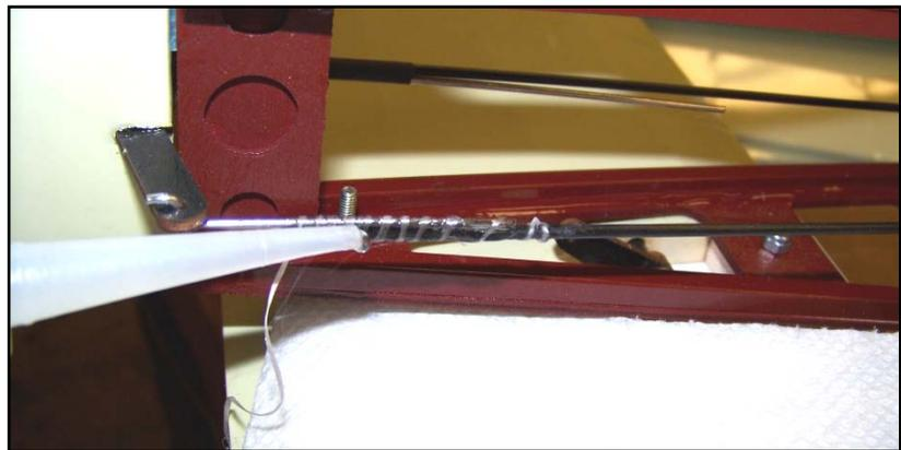
The horizontal stabilizer is held to the fuselage with machine screws and lock nuts. As I tightened the screws I felt like the nut was compressing the wood too much so I placed a washer under the head of both screws. Simple and inexpensive but again makes me feel better.
