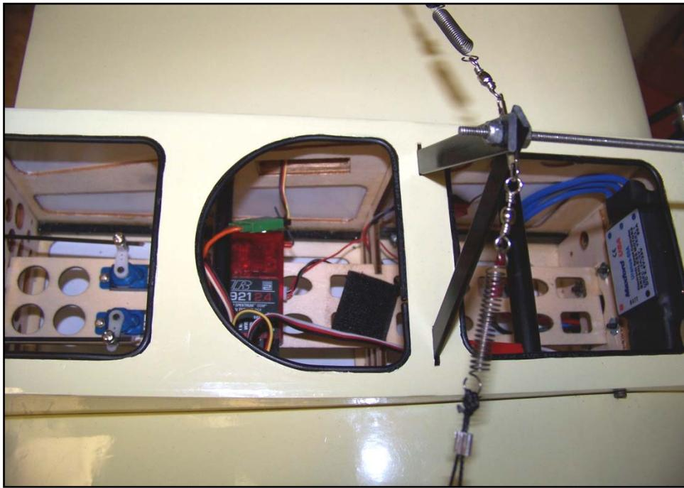
The upper wing-wire-mounting braces have a 4 3/4 inch metal rod between them for attachment of the wires. The one in the kit was not threaded properly on one end. For expediency, I used a piece of 4-40 all-thread and nuts which worked just fine but I have talked with Maxford USA and they would have gladly replaced the part had I called.
