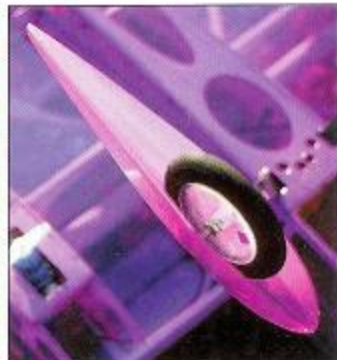
Micro receiver mounts under canopy for easy access. Note fine laser-cut woodwork with ample lightening holes cut wherever possible for weight savings. PVC wheel pants and cowl contribute to Spirit 3D's great appearance and low all-up weight.
