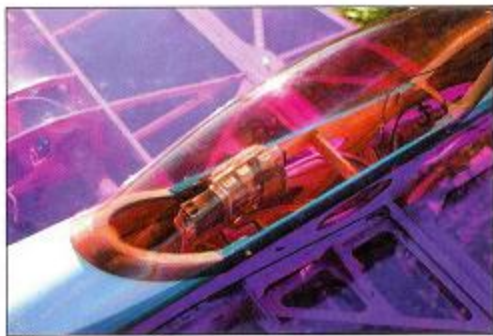
Micro receiver mounts under canopy for easy access. Note fine laser-cut woodwork with ample lightening holes cut wherever possible for weight savings. PVC wheel pants and cowl contribute to Spirit 3D's great appearance and low all-up weight.
