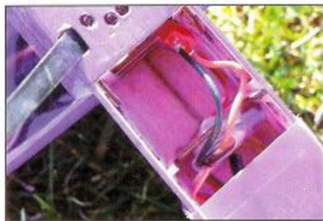
Easy access to ESC and battery is through hatch in chin compartment, just ahead of carbon fiber main gear.
