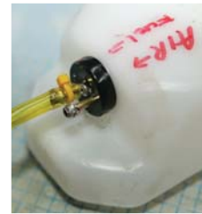
The gas tank with custom fastener
