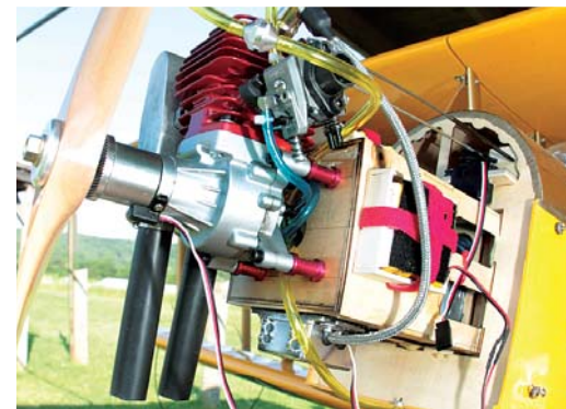
Because the plane needed nose weight, the ignition and receiver battery (not visible) were mounted on the engine box.
