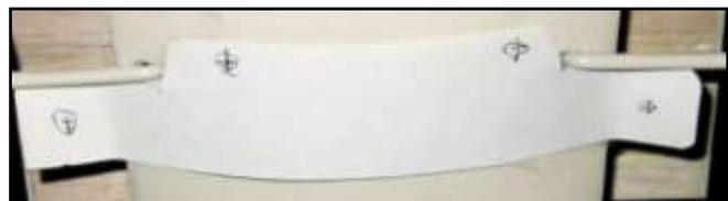
Position the retainer between the rear landing gear crossmember and the two lower wing panels, with two of its mounting holes behind the landing gear crossmember so that it covers the slot in the bottom of the fuselage and secures the main landing gear's rear cross-member and wooden retainer and with its remaining two holes extending out onto the lower wing panels.
