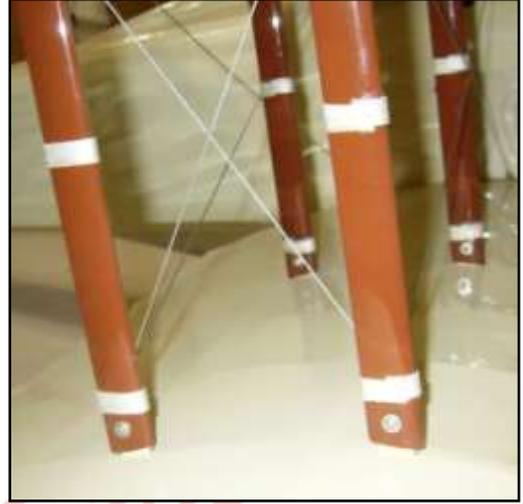
24. Connect the clevis end of the wires to the wing-wire anchors nearest the nose.
