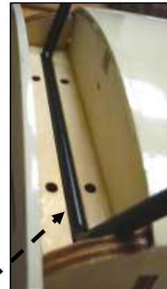
3. Press the landing gear's front crossmember into its mounting slot. Use the supplied metal straps, 5/8-inch machine bolts, and pre-installed blind nuts to secure the main landing gear's front crossmember to the fuselage.
