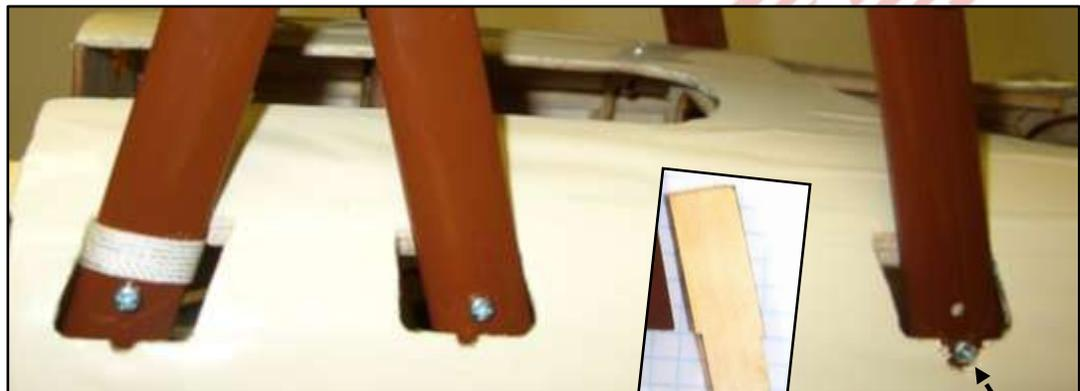
5. Using the lower wing as a reference, test-fit the cabane struts to align the upper wing's center section at "0-0" with the lower wing.
