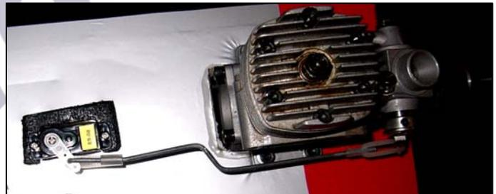
8. Assemble your fuel tank's vent and clunk lines in the stopper and secure the stopper in your fuel tank's opening.
