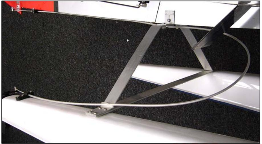
18. The rudder is attached to the hinge assembly with one hex bolt and nut; do not restrict the rudder's ability to LIFT (tilt up) by overtightening this bolt. Apply thread lock compound or CA adhesive to the threads at the outside end of the nut.
