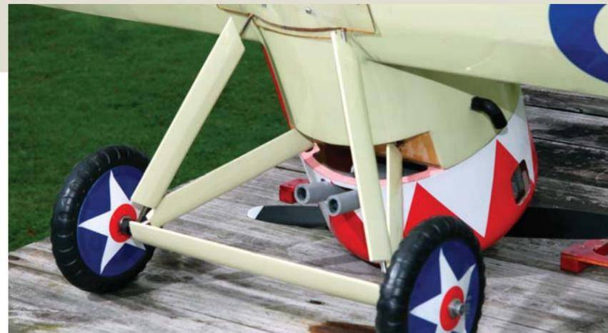
Wing support frames make wing removal and storage easy.
