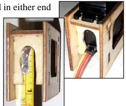
23. Assemble the provided **fuel tank** (i.e., open the 'stopper' for the vent and clunk lines, add the included short length of fuel tubing to attach the clunk to the clunk line, and use the included screw to seal the fuel tank's opening). Attach clunk and vent fuel lines to the outside of the tank, and insert the tank into the nose from the opening under the wing-saddle.
