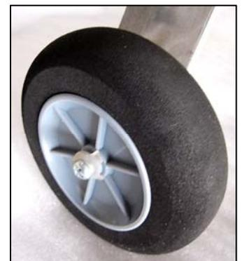
43. Tighten a supplied self-locking nut onto the remaining exposed threads at the inside of each axle bolt, secure the axle bolt against vibration by applying a drop of thick CA adhesive to the exposed threads at each self locking nut, and return the airplane to its 'right side up.'
