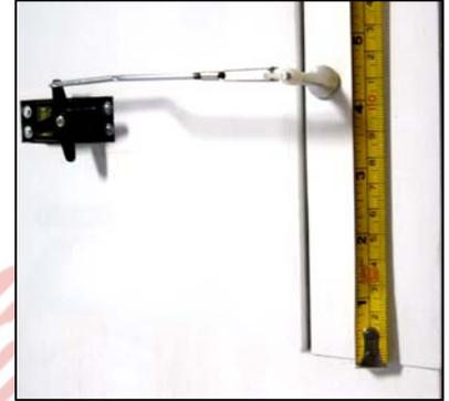
17. Using the pre-formed Z-bends and the supplied clevises, attach the 4-inch long **aileron pushrods**.
