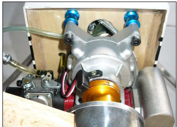
32. With the throttle servo in position, attach the **throttle servo's mount** to the inside of the fuselage with 5-minute epoxy.
