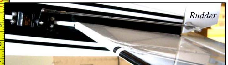
14. Connect a **12-inch servo-wire extension** to each of your aileron servos. Secure each connection with an optional "servo extension safety clip" and use masking tape and the provided string to pull each servo extension through its wing panel and out the hole near the wing root.
