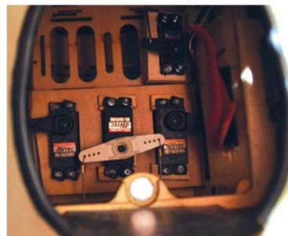
The Hitec servos are accessible through the large cockpit opening. Note the magnet, used to secure a cover plate in place.
