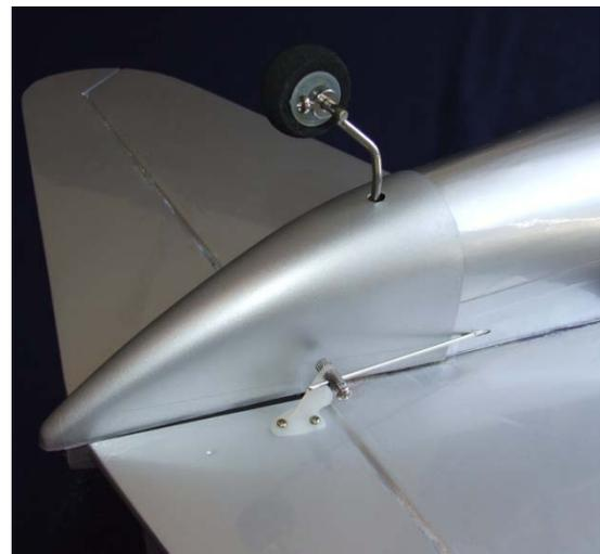
preinstalled guide tube on the **left** side of the fuselage and through the pushrod connector on the elevator control horn. Put the Z bend of the pushrod through the **inner** hole of the arm on the left servo. Center the servo and the elevator, then tighten the pushrod connector.
