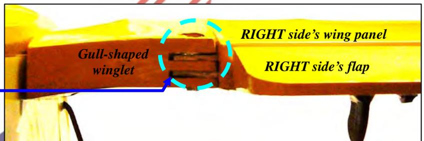
48. Insert a supplied 1/2-inch-long machine bolt into the hole in the top of the gull-shaped winglet. Press the bolt fully through all of the wing panel's metal hinge projections and the winglet's slotted openings until the end of the bolt becomes visible at the bottom of the wing.
