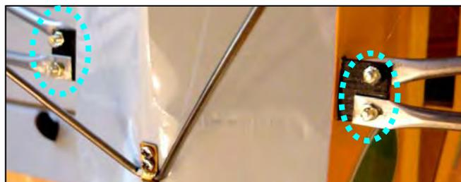
57. Use a 'dot' of hot-melt glue to attach the diagonal braces at each side of the vertical and above the horizontal stabilizer.....
