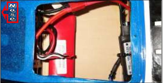
7. With the motor's three wires connected to ESC's three wires, connect the ESC's BEC/throttle connector to your receiver's throttle channel, and check the motor's rotation direction ...
