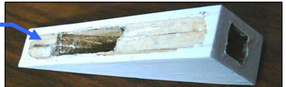
25. Slide the elevator pushrod fairing over the elevator pushrod's housing, and use 5-minute epoxy to permanently attach the elevator pushrod fairing to the top of the horizontal stabilizer.
