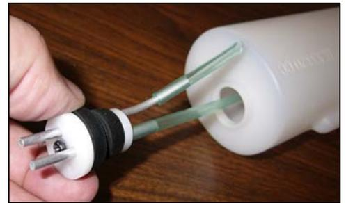
39. Connect the tank's 'clunk' line to the carburetor and the 'vent' line to the muffler. If you set up your Neptune for electric power,
