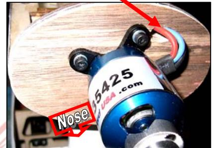
5. Check the engine/motor pod's left/right angle to ensure the propeller is at zero degrees by gently twisting the carbon fiber tube within its mounting hole. Once you are content with the propeller's angle, apply 5-minute epoxy mixed with some fibers from a cotton ball to secure the pod into the fuselage at the base of the carbon fiber tube and to fill the small gap between the carbon fiber tube and the top of the fuselage.
